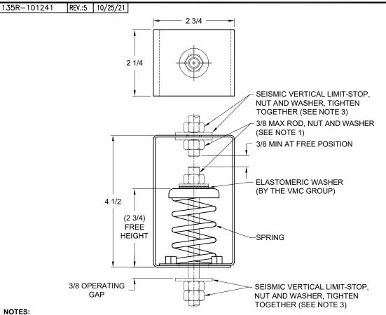
TYPE HS-1B SPRING HANGERS FOR 1" NOMINAL DEFLECTION DEFLECTION RATED LOAD SPRING RATE SPRING **HANGER** (LBS) **COLOR CODE** (IN) (LB/IN) HS-1B-20 DK BLUE 20 1.25 HS-1B-35 35 1.17 30 BLACK HS-1B-50 50 1.11 45 RED HS-1B-70 70 DK GREEN 0.88 HS-1B-85 85 0.81 **GRAY**
